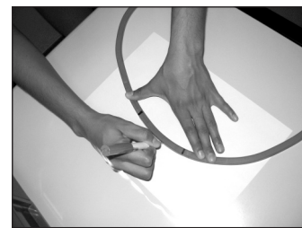
Figure 3 Transference of the curvature measurement onto paper.
