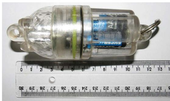
**Figure 1.** Model of electric fishing light commonly used by southern Brazilian pelagic longline fleet.
