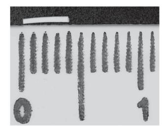
**FIGURE 1 -** Dexamethasone-loaded PLGA implant (weight:  $6.0 \pm 0.1$ mg; length:  $4.0 \pm 0.1$  mm; diameter:  $1.0 \pm 0.05$  mm).
