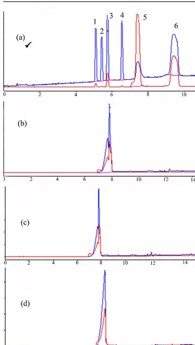
**Figure S4** - Effect of sample pH on analysis,  $\lambda=214$  nm (blue line),  $\lambda=257$  nm (red line), a) pH 7.0 b) pH 9.0 c) pH 11.0 d) pH 5.0 e) pH 3.0, Conditions: Hydrodynamic injection  $P_{inj}=50$  mbar, Separation Voltage=30 kV, Capillary diameter: 75  $\mu\text{m}$ , BGE: 75  $\text{mmol L}^{-1}$  Sodium borate (pH: 8.0) buffer-15% ACN, Peaks: 1) DEX 2) EPH 3) CHL 4) PSE 5) 4-AP 6) PAR
