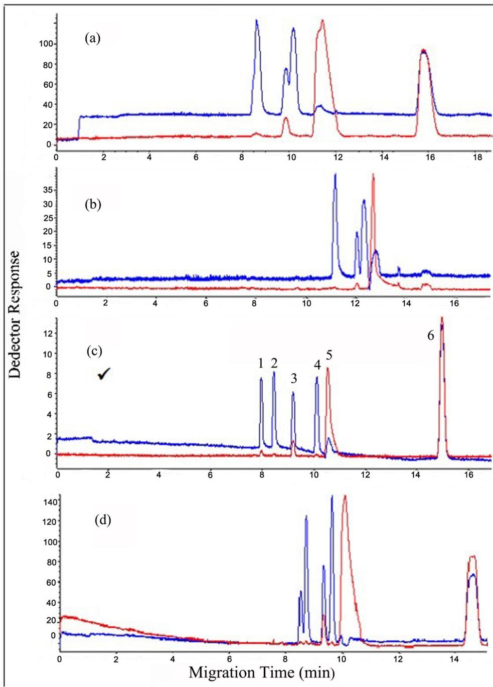
**Figure 2** - Effect of buffer concentration on analysis  $\lambda=214$  nm (blue line),  $\lambda=257$  nm (red line), Buffer: NaBorat (pH 8), Buffer concentrations: a)25 mM b)50 mM c)75 mM d)100 mM, Conditions: Capillary diameter 50  $\mu$ m, Hydrodynamic injection  $P_{inj}=50$  mbar, Isolation Voltage=30 kV, T: 20°C, Peaks: 1)DEX 2)EPH 3)CHL 4)PSE 5)4-AP 6)PAR
