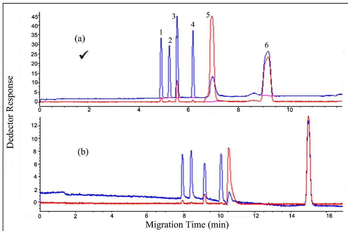
**Figure S2** - Effect of capillary diameter on analysis  $\lambda=214$  nm (blue line),  $\lambda=257$  nm (red line), Capillary diameters: a) 75  $\mu\text{m}$  b) 50  $\mu\text{m}$ , Conditions: Hydrodynamic injection  $P_{inj}=50$  mbar, Separation Voltage=30 kV, T: 20°C, BGE: 75 mmol L<sup>-1</sup> Sodium borate (pH: 8.0) buffer-15% ACN, Peaks: 1)DEX 2)EPH 3)CHL 4)PSE 5)4-AP 6)PAR
