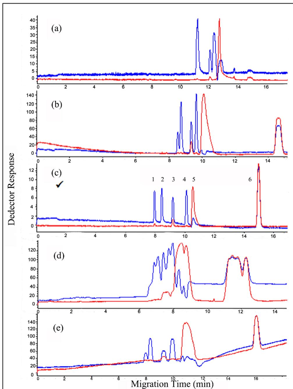
**Figure S1-** Effect of percentage of organic solvent on analysis  $\lambda=214$  nm (blue line),  $\lambda=257$  nm (red line), Percentages of acetonitrile: a)30% b)20% c)15% d)10% e)0%,
