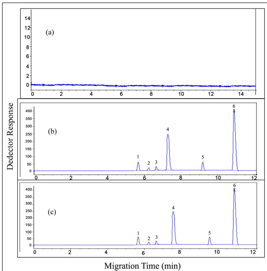
**Figure 3** - Electropherograms at  $\lambda=192\text{nm}$ , a)BGE solution, b)Standard solutions of DEX, EPH, CHL, PSE, 4-AP, PAR, respectively, c)Solution containing pharmaceutical preparation (Gripamol tablet) and impurities, Conditions:  $t_{inj}=10\text{ s}$ , Hydrodynamic injection  $P_{inj}=50\text{ mbar}$ , Isolation Voltage=30 kV, Capillary diameter: 75  $\mu\text{m}$ , BGE: 75 mM NaBorat (pH: 8.0) buffer-15% ACN,  $T=30^\circ\text{C}$
