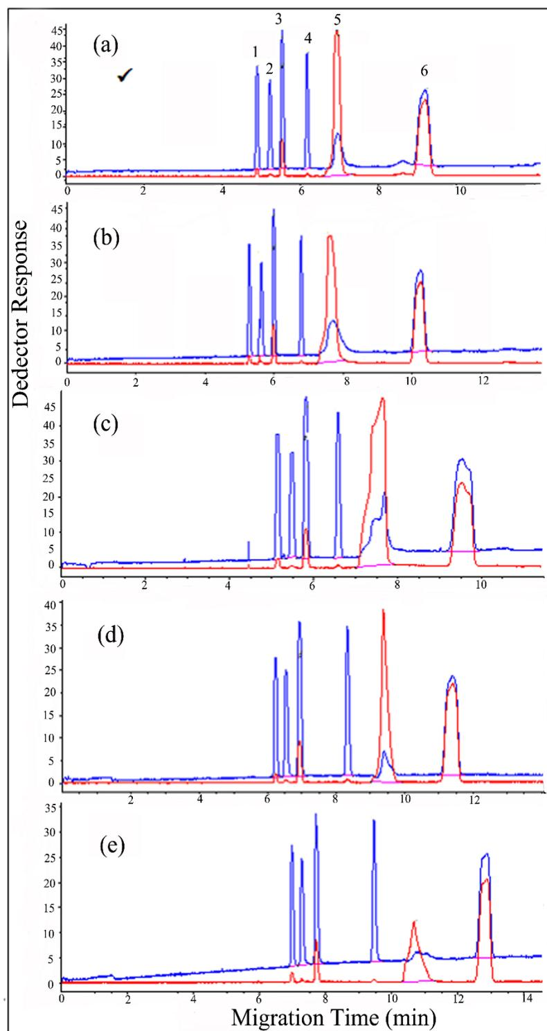
**Figure S3** - Effect of temperature on analysis  $\lambda=214$  nm (blue line),  $\lambda=257$  nm (red line), Temperatures: a)30°C b)25°C c)20°C d)15°C e)10°C, Conditions: Hydrodynamic injection  $P_{inj}=50$  mbar, Isolation Voltage=30 kV, Capillary diameter: 75  $\mu\text{m}$ , BGE: 75 mmol L<sup>-1</sup> Sodium borate (pH: 8.0) buffer-15% ACN, Peaks: 1)DEX 2)EPH 3)CHL 4)PSE 5)4-AP 6)PAR
