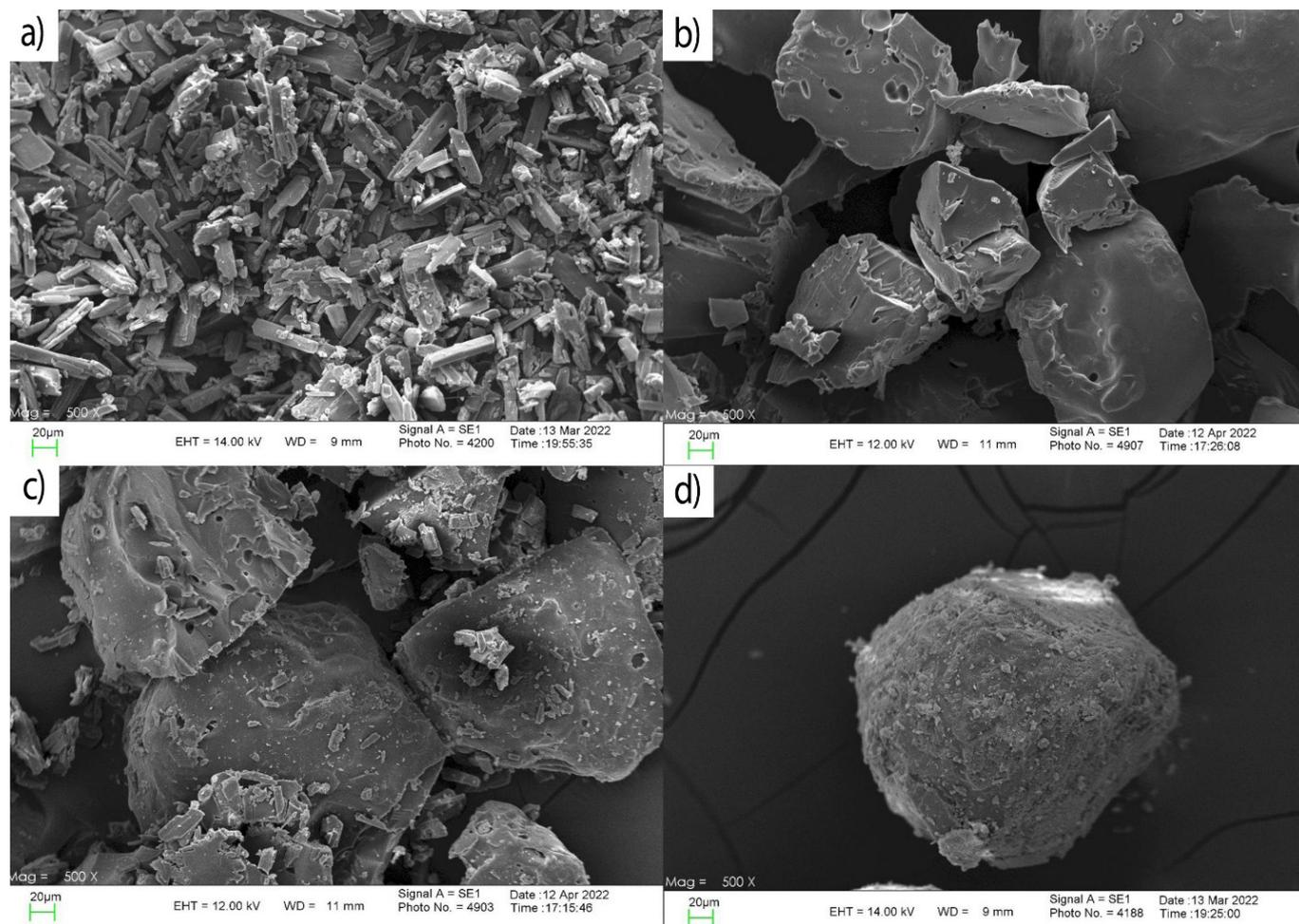
**FIGURE 6** - SEM images of a) STZ, b) Soluplus®, c) STZ-PM and d) STZ-SD.
