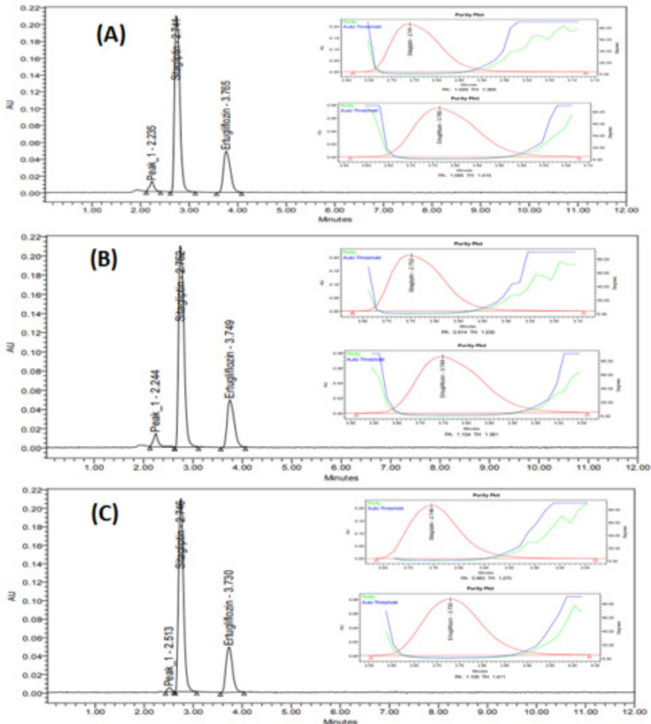
FIGURE 5 - HPLC chromatograms of drugs under stress conditions: acid (A), base (B), oxidative (C) and peak purity plots.
