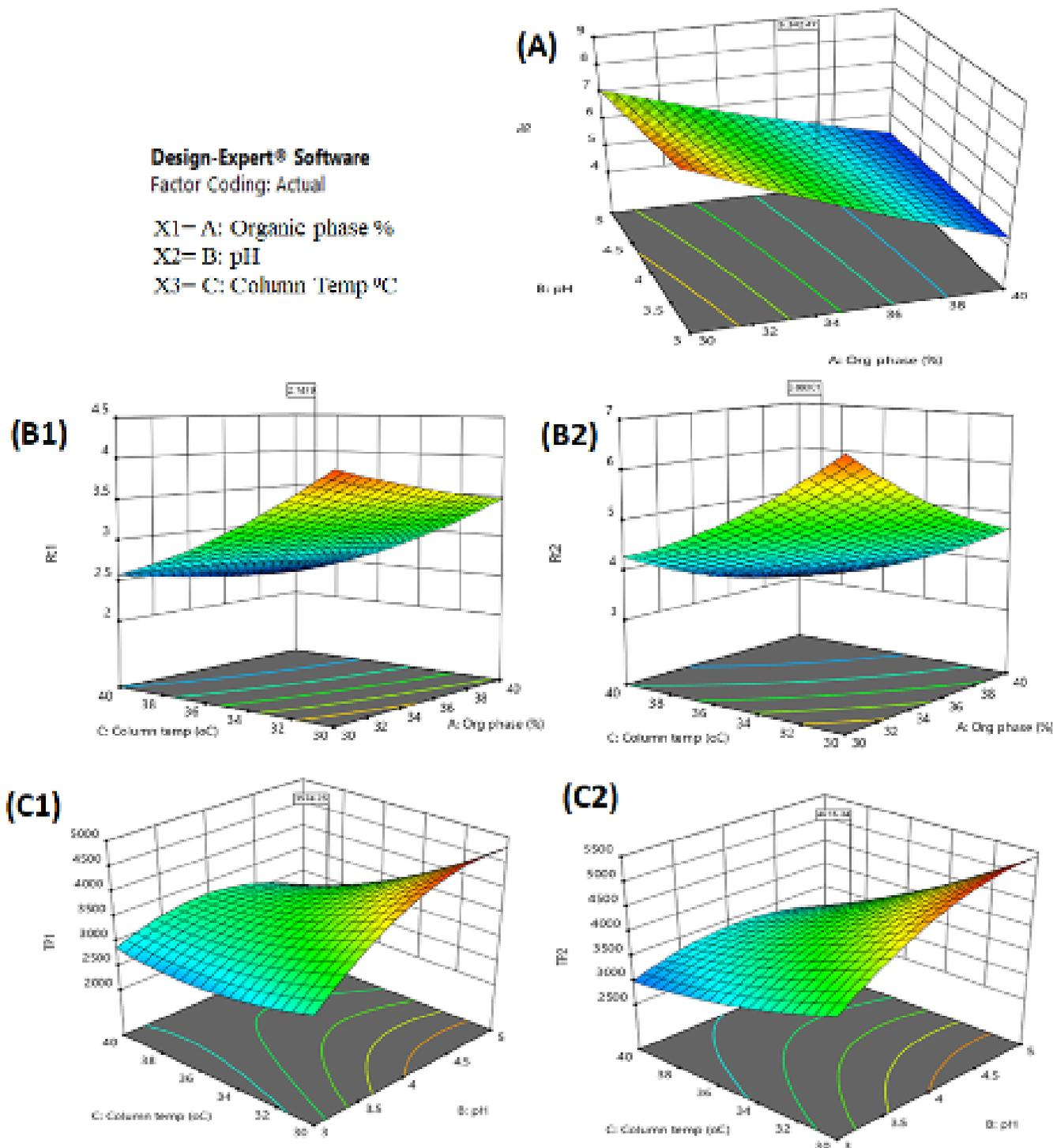
**FIGURE 2** - Response surface plots: Resolution (A); retention time of SIT (B1); retention time of ERT (B2); theoretical plates of SIT (C1); theoretical plates of ERT (C2).
