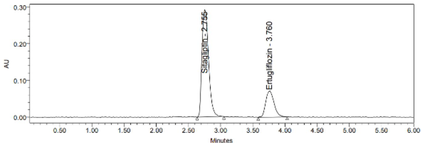
**FIGURE 6** - HPLC chromatogram of formulation (Steglujan<sup>®</sup> tablets) solution.
