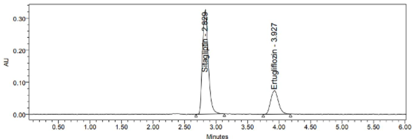
**FIGURE 4** - HPLC chromatogram under optimised conditions: mobile phase acetonitrile:acetate buffer, pH 4.4 (36:64 % v/v) at flow rate 1 mL/min, column temperature 37 °C.
