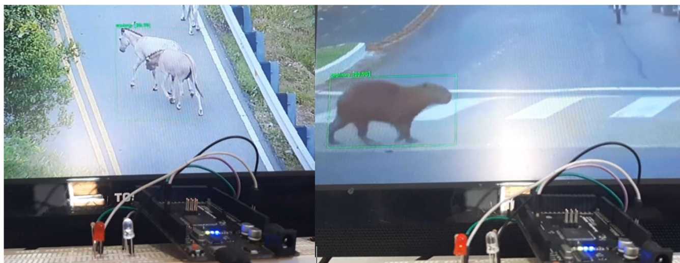
Figure 8 – Light alert for true-positive detections. Left frame – white LED blinks for equidae class detection; Right frame – red LED blinks for capivara class detection.
