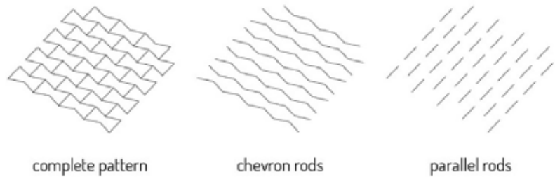
Figure 5: Schematization of rod typologies. The re-entrant honeycombs pattern is defined by two types of rods: the indented elastic rods called the Chevron rods and the inelastic rods which are known as the parallel rods
