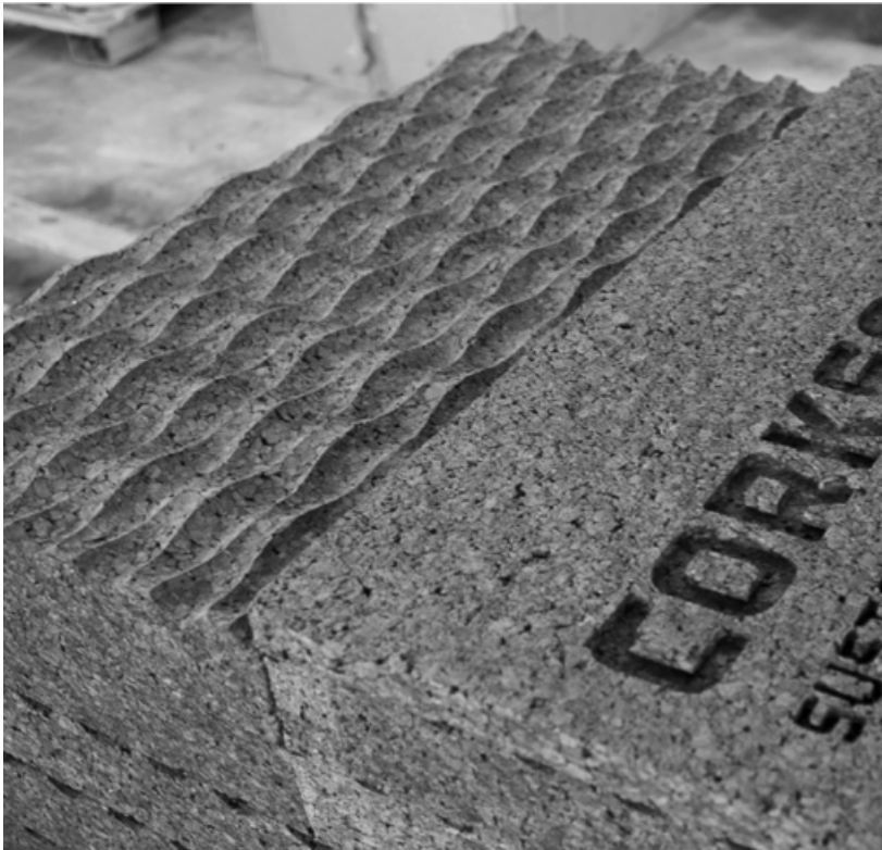
Figure 1 : CNC milled insulation cork boards. © 2014 Filipe Brandão
