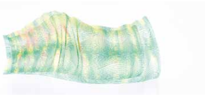
Figure 13: Curvature analysis of wefts in the digital model. The more the rattan is bent the more force is locally applied on the wooden warps, increasing the friction between the warps and wefts
