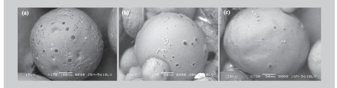
FIGURE 1 - SEM photomicrographs of floating microspheres of verapamil hydrochloride.
