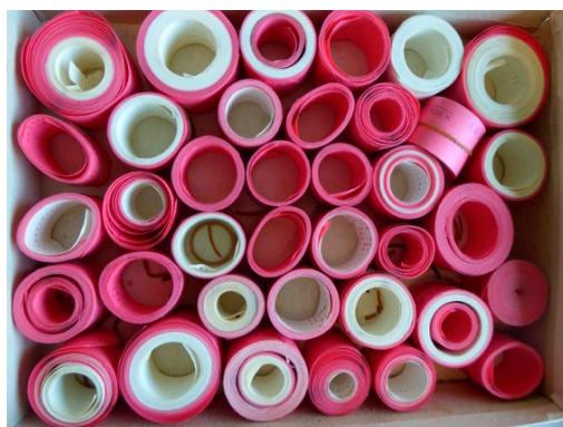
Fig. 2. Perforated tapes used on the NCR Elliott 4100 computer, Porto, Laboratory of Automatic Calculation (LACA-FCUP), c. 1968.
